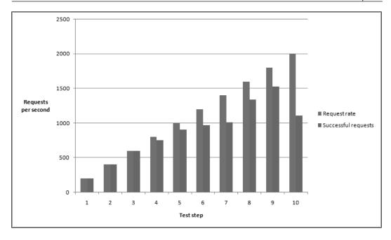
As you can tell from the graph, this test server supports up to 600 requests per second without a loss. Past this limit, some connections get dropped as Nginx cannot handle the load. It stills gets up to over 1,500 successful requests per second at step 9.
