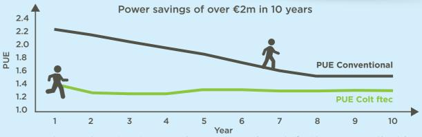
Based on a growth scenario, maximum power of 1.5MW, energy cost of 10c per kW/hr with 3% per annum uplift. Colt ftec achieves a target PUE of 1.21 after 4 years, conventional build PUE of 1.5 in eighth year.
